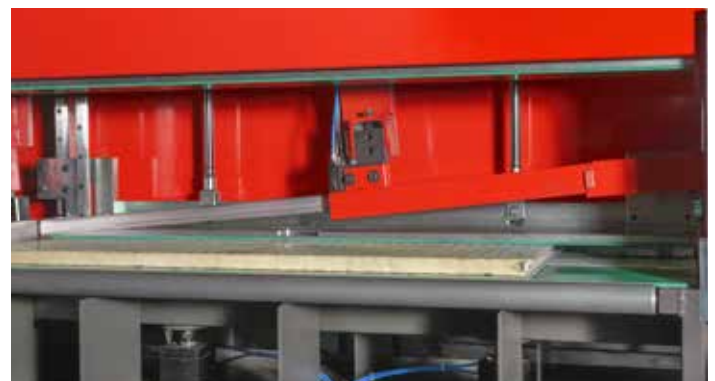
Pattino guidalama mobile – Movable blade guide
