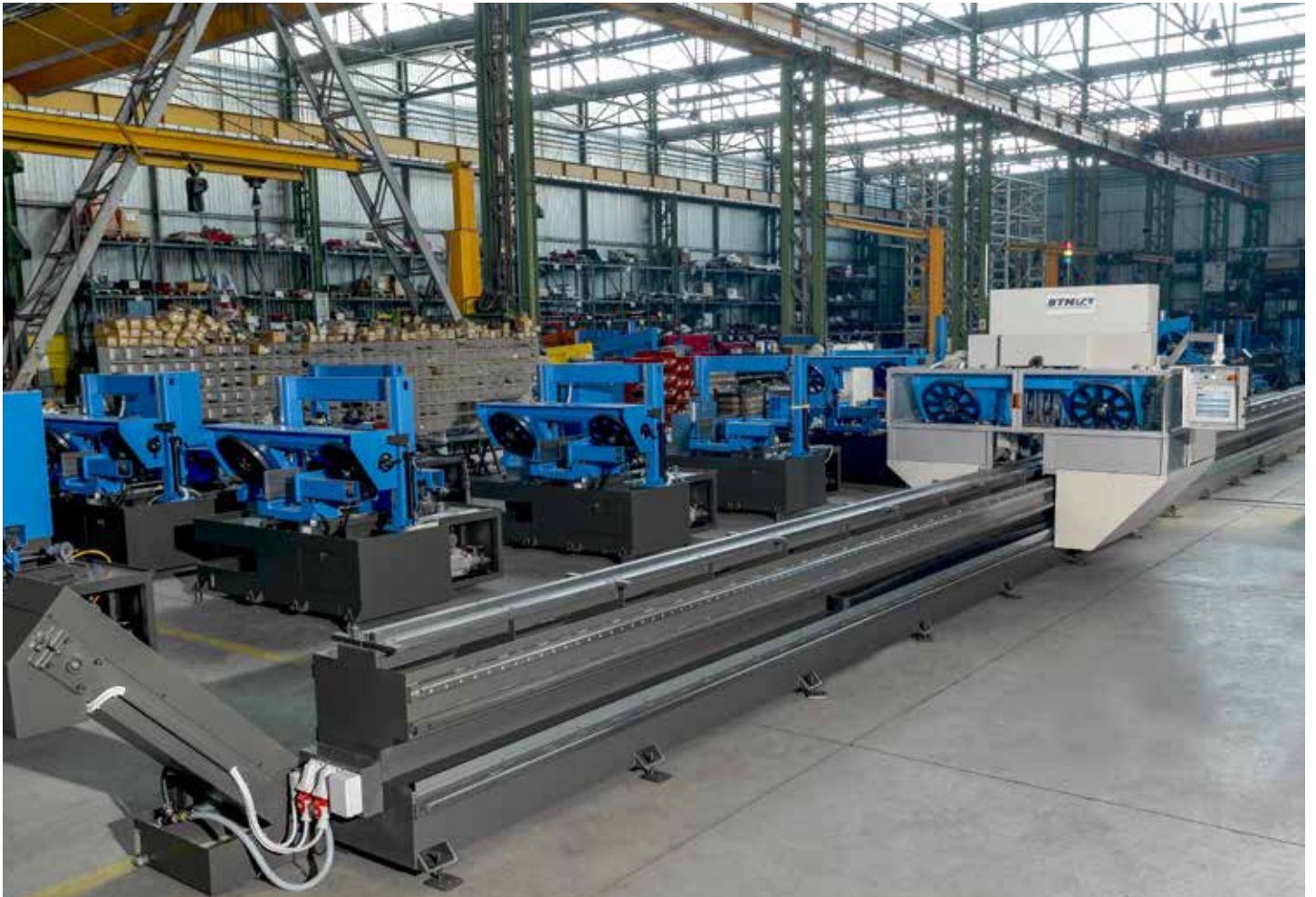
Impianto speciale per taglio e foratura binari con diametro massimo 40 mm Special system for cutting and drilling tracks with a maximum diameter of 40 mm
